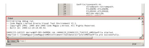
The red high-lighted window shows the output generated during the execution of a job within the VTE. This output is the same as the the EresiaOutput.txt file in the job window.
